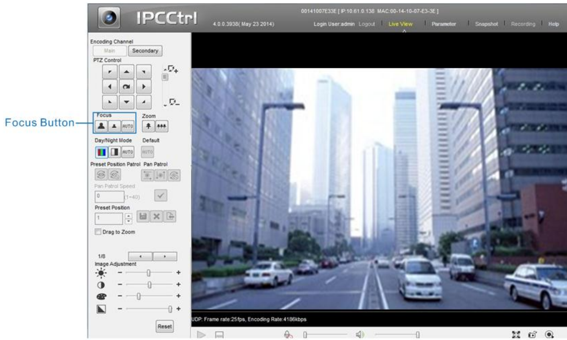
Picture 3-5 Electrical Focus
